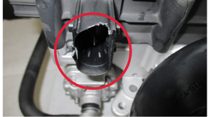
Broken plug connector, damaged by unprofessional disassembly
