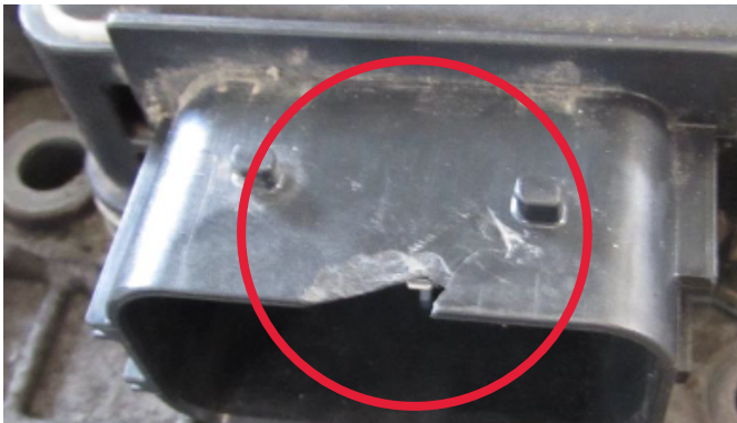
Broken plug connector, damaged by unprofessional disassembly
