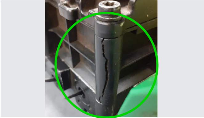
Cracked ECU corners
